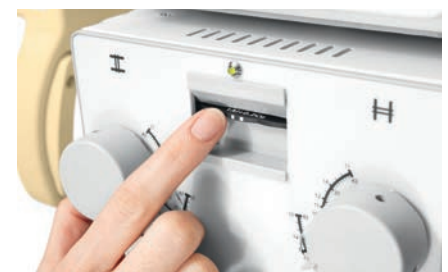
Built-in spectral filters for exceptional X-ray dose management
